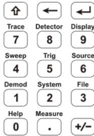
Figure 3-6 Shift key and function hardkeys
