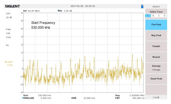
As expected, the frequency range is crowded with broadcast signals. It next needs to be figured out, if the emissions of the DUT are above or in between with respect to amplitude.
