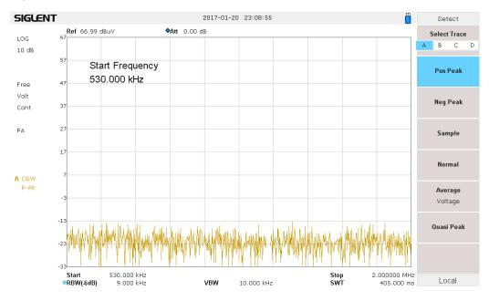
The displayed noise floor with this settings is approximately at  $-20 dB\mu V$  which is impressive for a Spectrum Analyzer of this class. However it needs to be considered that the frequency range of interest is crowded with AM broadcast signals which are likely to be picked up.
