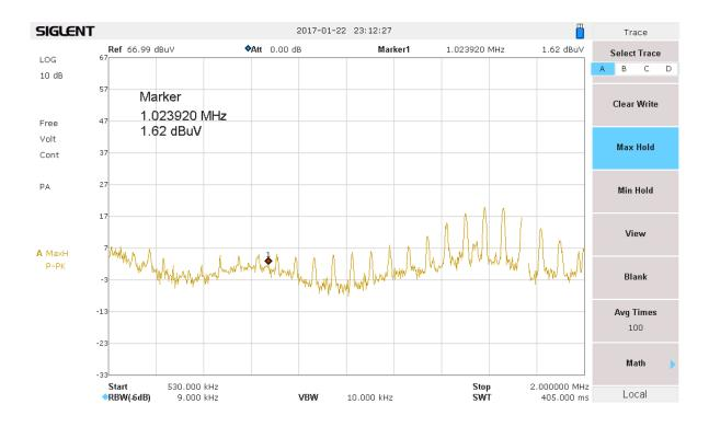
In order to get a clearer picture, the span of the Spectrum Analyzer was reduced and set in between two adjacent broadcast channels.
