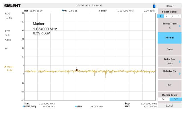
The modification gave a 12 dBµV reduction of the radiated emissions level at the investigated frequency.
