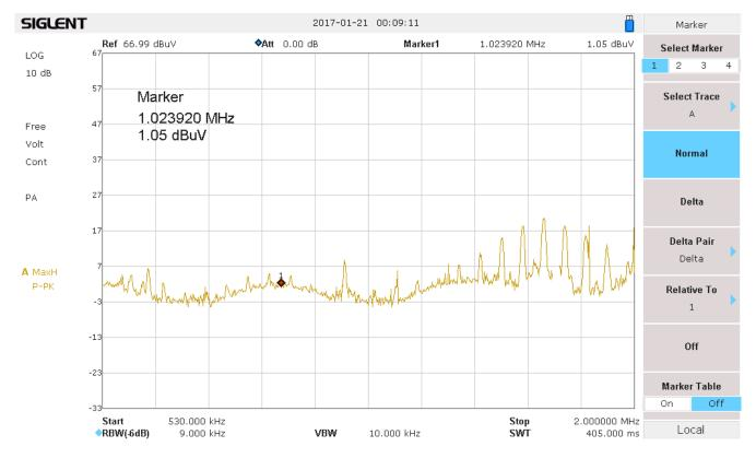
"Removing" the cable reduces the radiated noise at abpproximately 11 dBµV. Checking back with the customer turned out, that in fact not the cable was removed, but the two radar sensors were disconnected. This also explains why the relative amplitude of the spectrum "hills" are a bit different compared to the TEM cell measurement. The cable was set up straight in the anechoic chamber, whereas in the TEM cell it is coiled.
