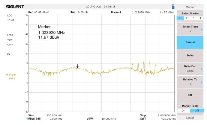
The "hills" visible in the measured spectrum nicely correlate with the plot of the measurement in the anechoic chamber, despite the presence of some peaks from AM broadcast signals. The amplitude measured in the TEM cell is approximately 20 dBµV lower compared to the amplitude measured in the anechoic chamber.
