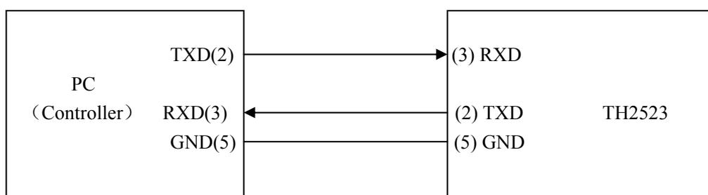
Figure 6-1 Connection of the instrument with PC
