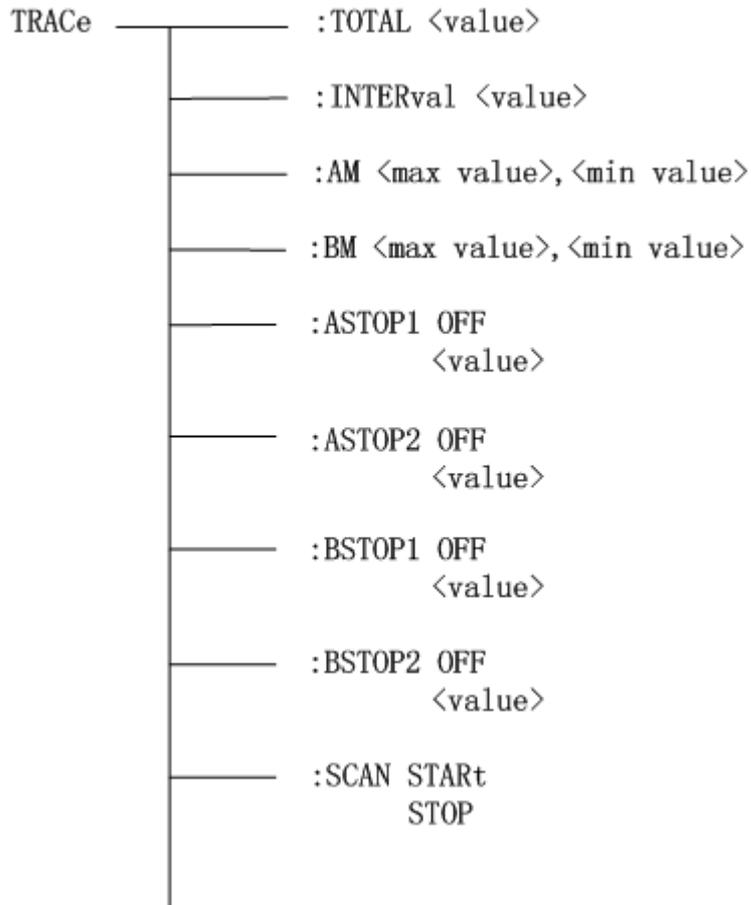
The :TRACe:TOTAL <value> command is used to set and return the total time of scanning.
