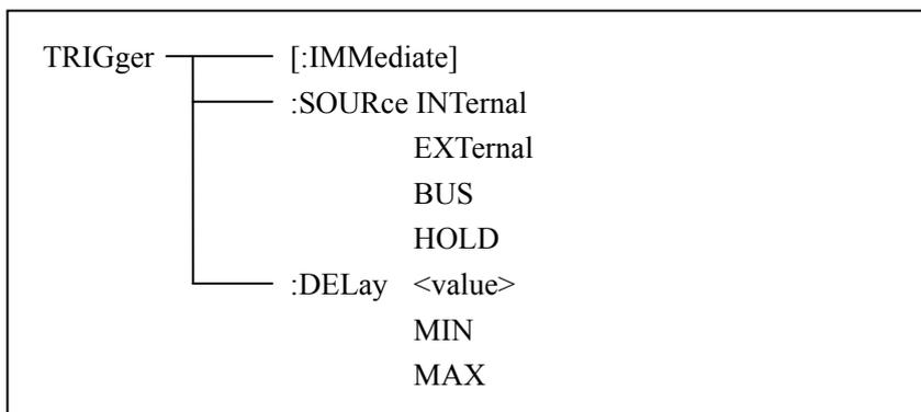
The :IMMEDIATE command triggers a measurement.
