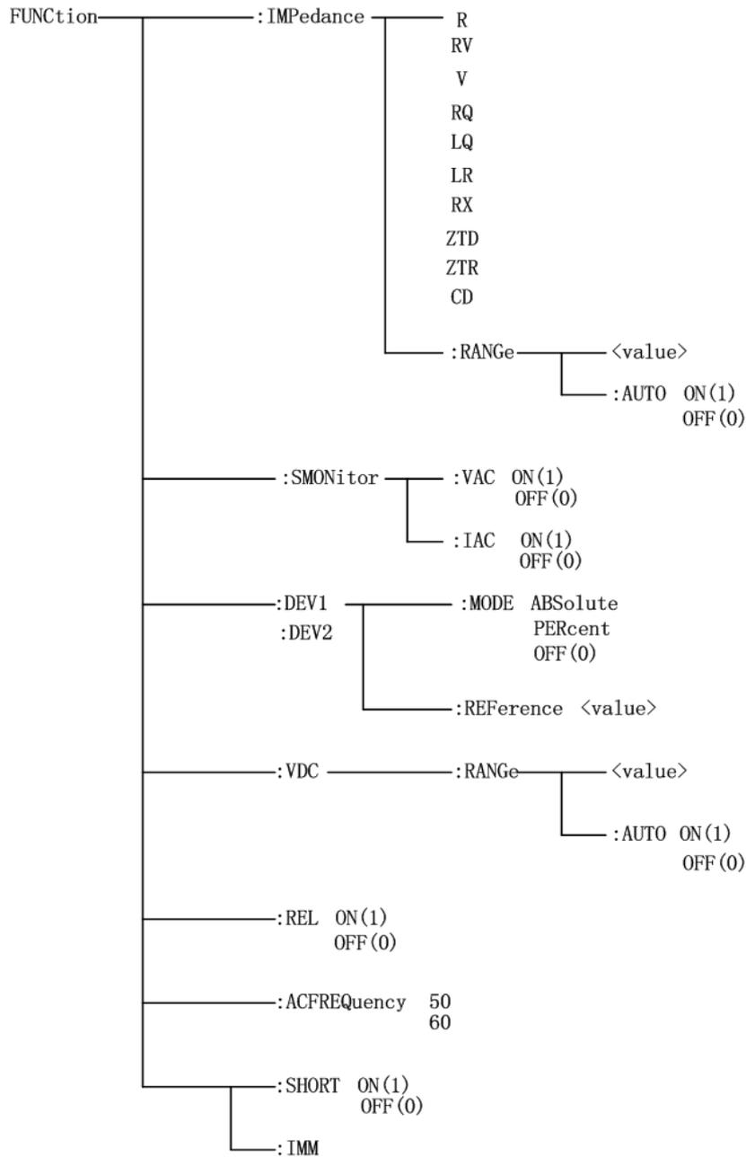
The :IMPedance command sets the “function” parameters.
