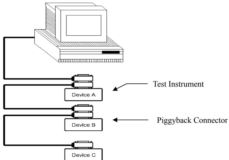
Figure 6-3 Typical GPIB System Interconnection for Double-piggyback Connector
