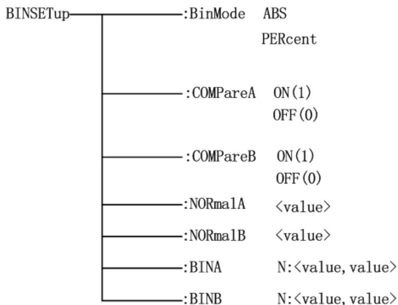
The:BINSETup:BinMode command set the bin compare mode. The:BINSETup:BinMode? query returns the current compare mode.
