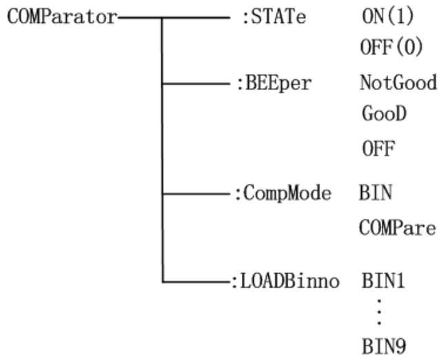
The [:STATe] command sets the comparator function ON or OFF.
