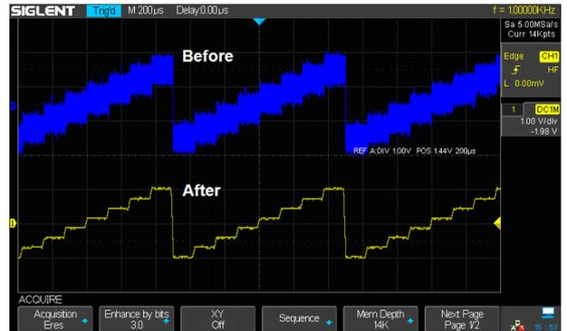
Eres mode can improve the SNR effectively, without the dependence on the periodicity of signal and stable triggering
