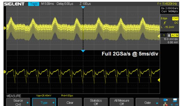
Using hardware-based Zoom technique and record length of up to 140Mpts, users are able to use a higher sampling rate to capture more of the signal, and then quickly zoom in to focus on the area of interest
