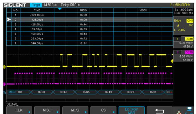
Displays the decoding through the events list. Bus protocol information can be quickly and intuitively displayed in table form
