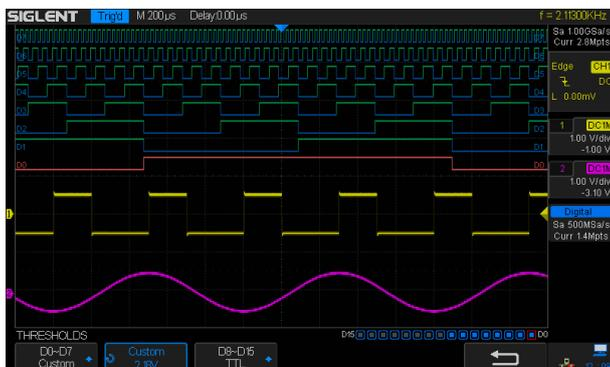
4 analog channels plus 16 digital channels enables users to acquire and trigger on the waveforms then analyze the pattern, simultaneously with one instrument.
