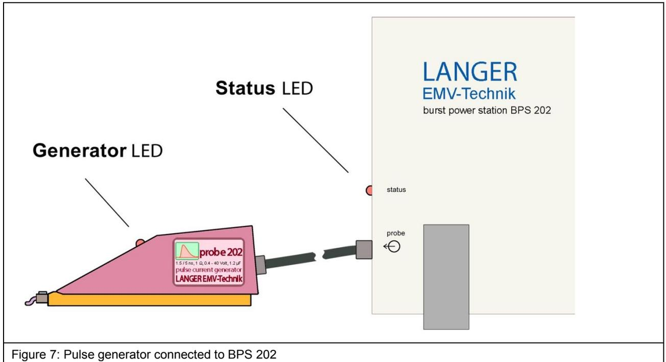
Figure 7: Pulse generator connected to BPS 202
