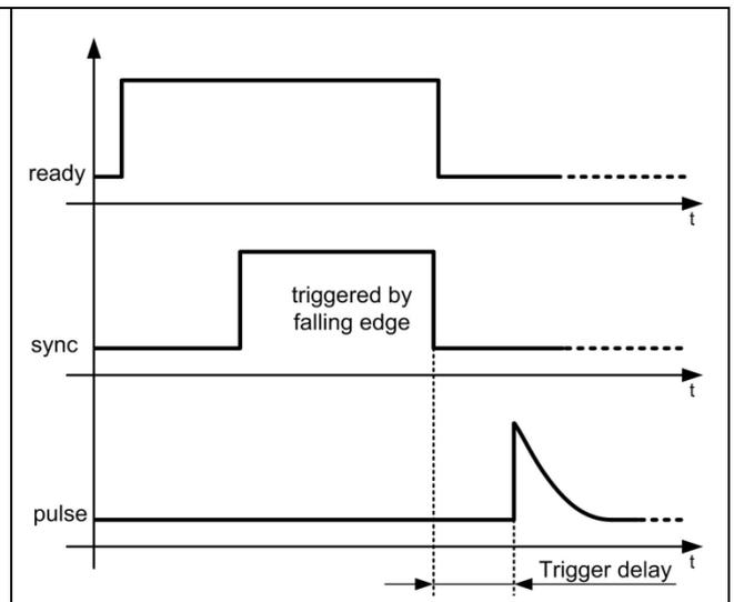
Figure 44: Signal sequence of external trigger mode, trigger on falling edge
