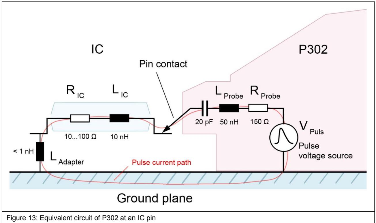
Figure 13: Equivalent circuit of P302 at an IC pin
