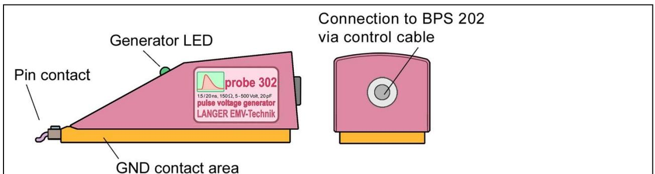
Figure 12: Schematic view from the side and back of P302
