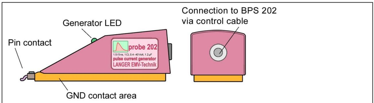
Figure 9: Schematic view from the side and back of P202
