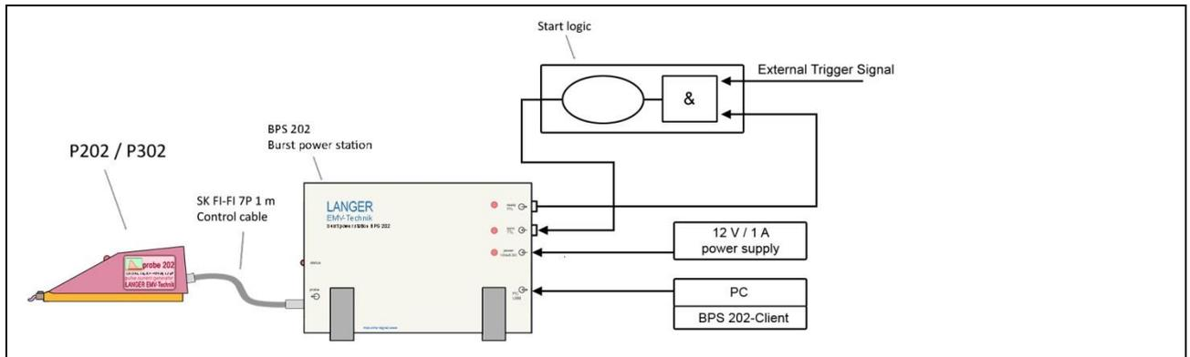
Figure 42 System set-up for external trigger event via BPS 202 sync TTL input
