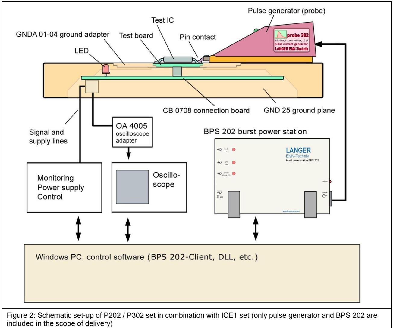
Figure 2: Schematic set-up of P202 / P302 set in combination with ICE1 set (only pulse generator and BPS 202 are included in the scope of delivery)
