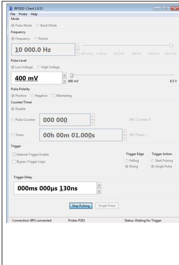
Figure 31: Trigger for **Pulse Mode**
