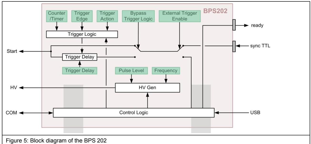
Figure 5: Block diagram of the BPS 202
