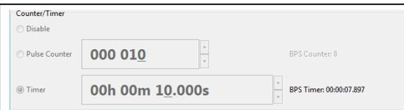
Figure 29: BPS Timer in Counter/Timer section
