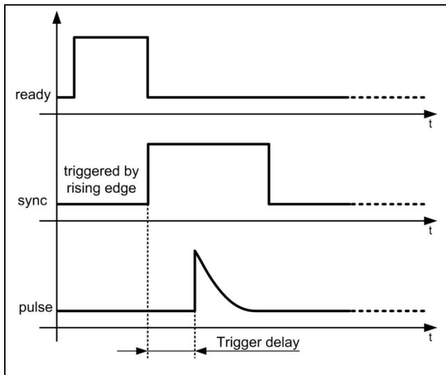
Figure 43: Signal sequence of external trigger mode, trigger on rising edge
