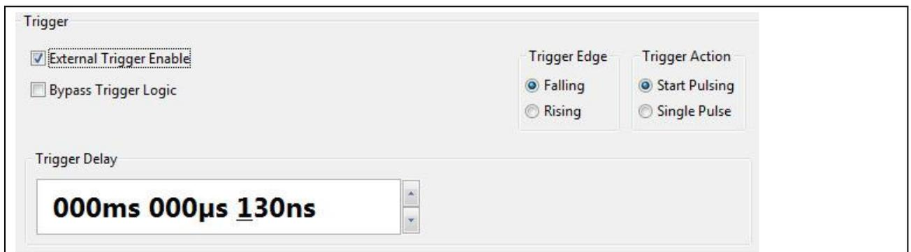
Figure 26: GUI section Trigger for operating mode pulse mode
