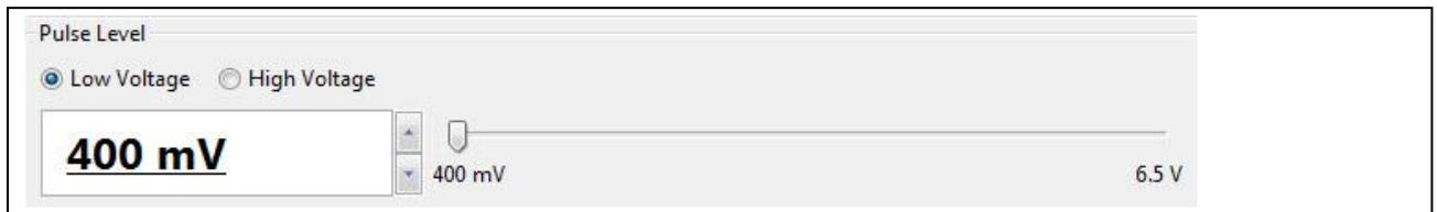
Figure 20: Setting of the Pulse Level with Low Voltage option selected
