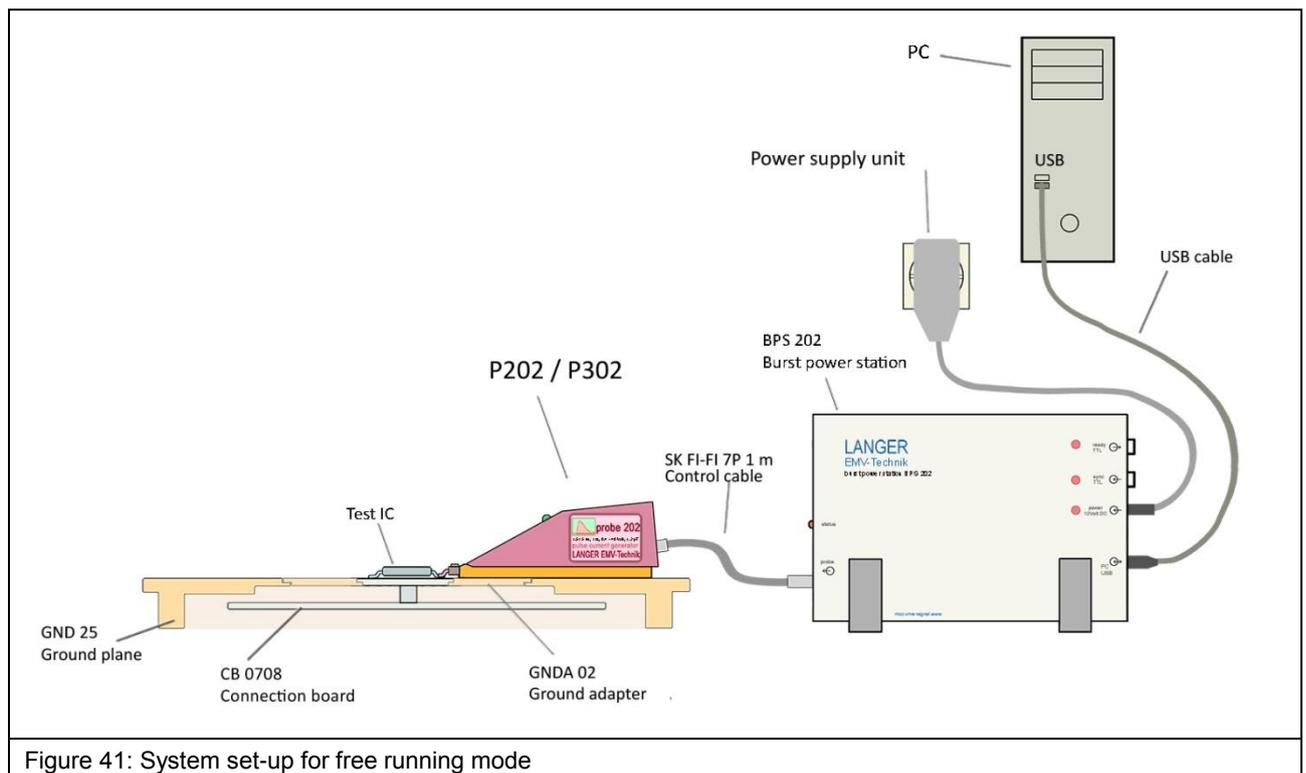
Figure 41: System set-up for free running mode
