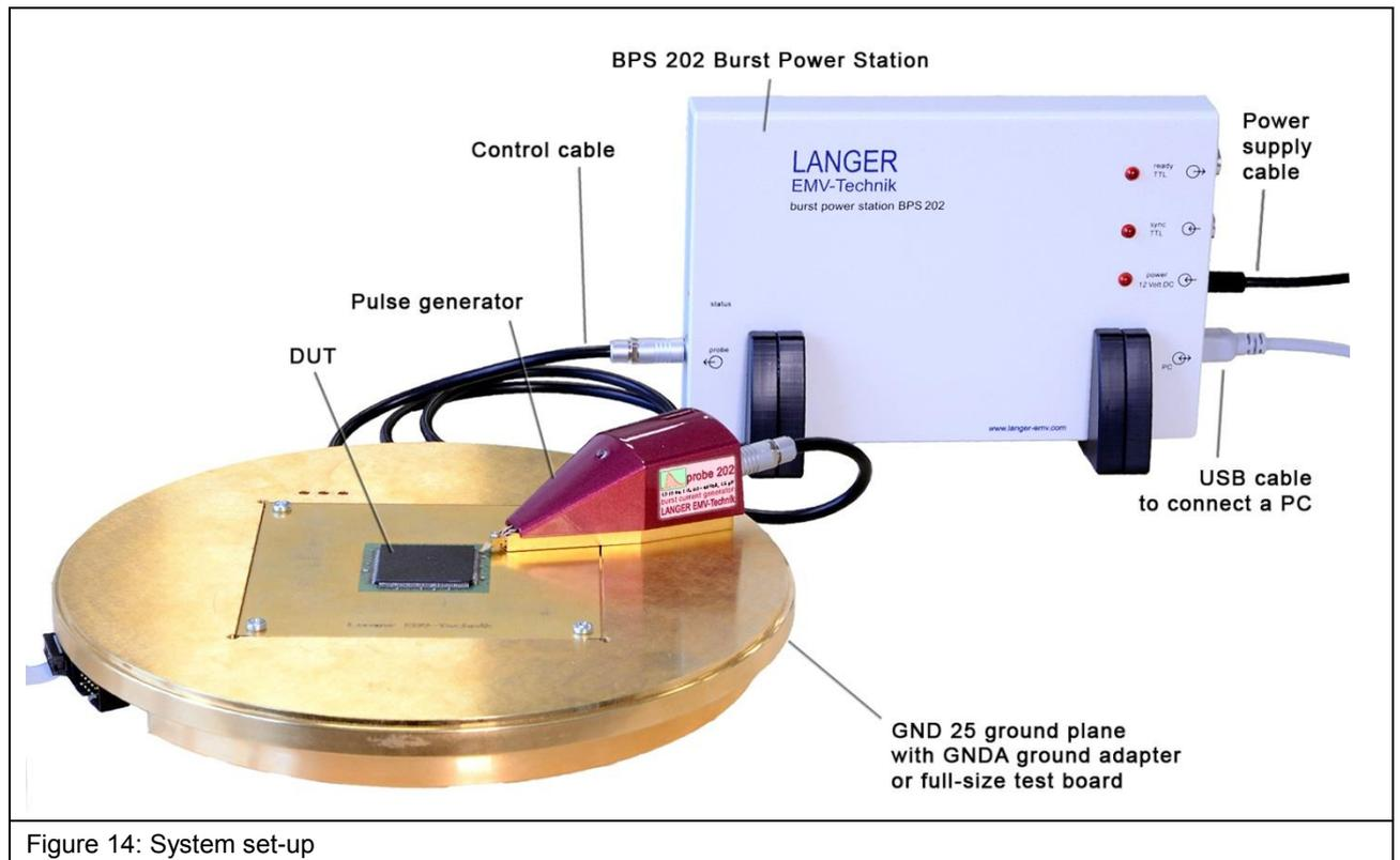
Figure 14: System set-up
