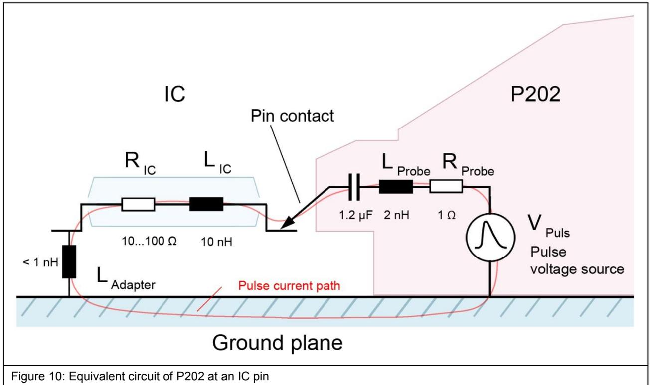
Figure 10: Equivalent circuit of P202 at an IC pin
