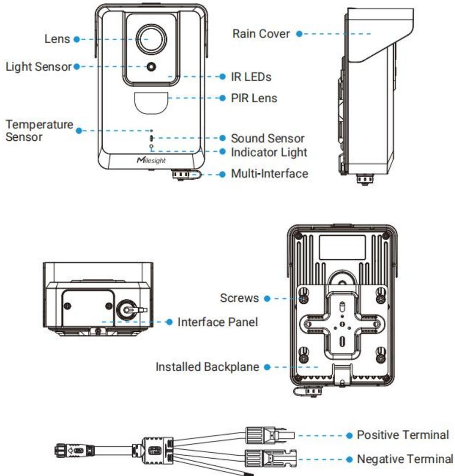
**Note:** The Positive Terminal of the solar panel cable needs to be connected to the Negative Terminal of the solar panel, and the Negative Terminal needs to be connected to the Positive Terminal of the solar panel.
