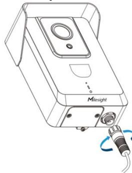
**Step 8:** Connect the device to the backplane that you've installed already and tighten the fixing screws. Then the installation is completed.
