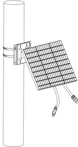
**Step 7:** Connect the solar panel to the Solar Charging Interface.
