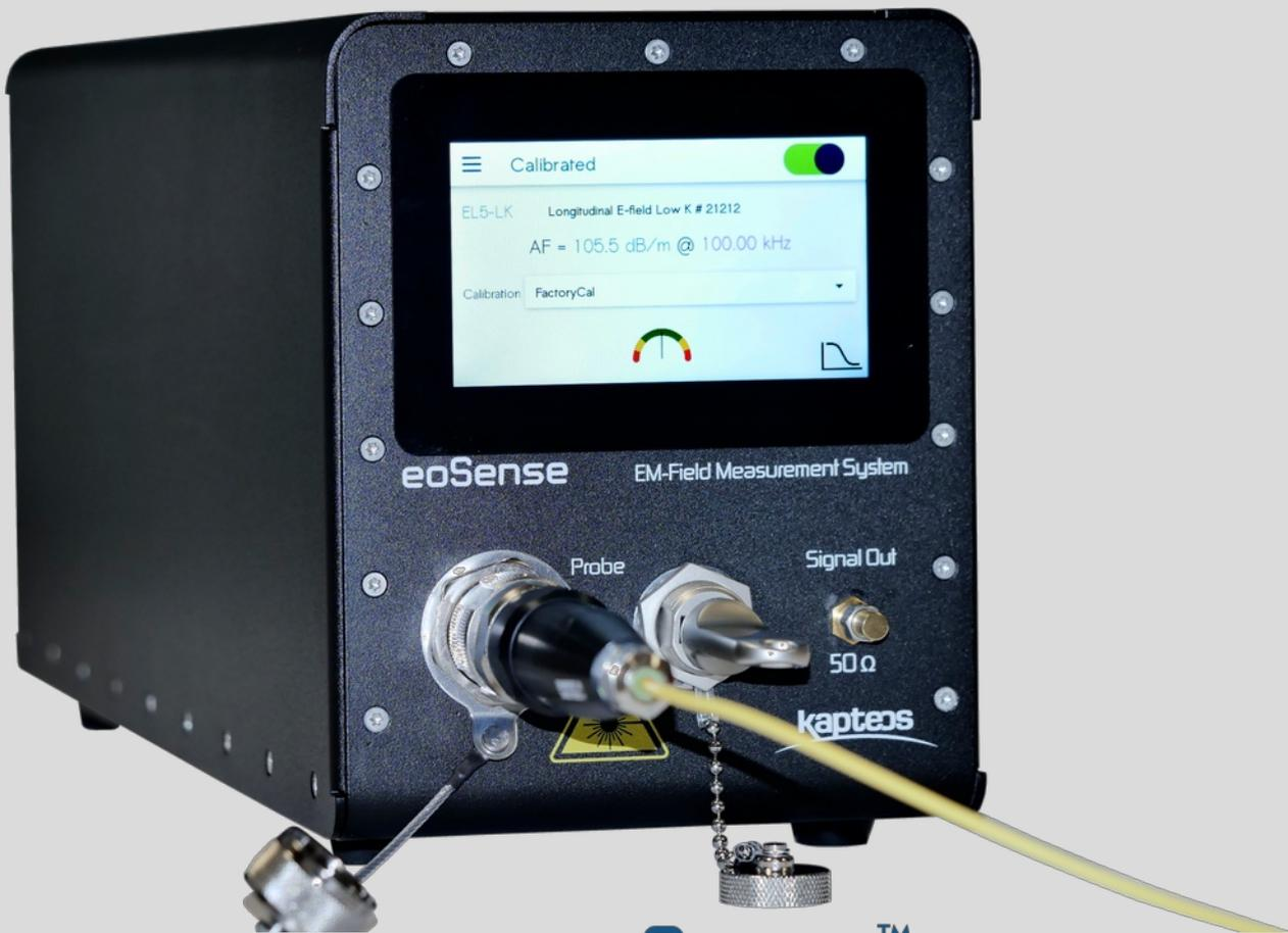
Optoelectronic converter **eoSense™** 4<sup>th</sup> generation
