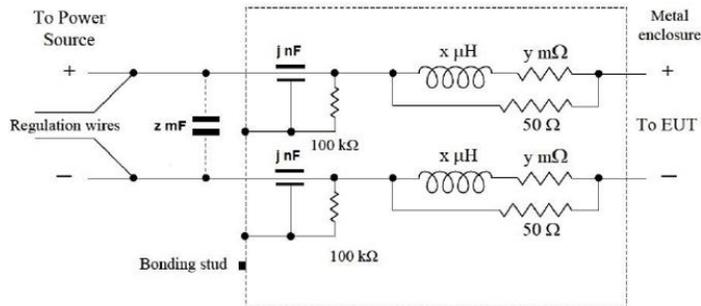
Figure 5-2: LISN schematic
