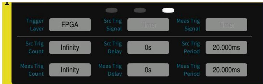
Figure 4-11 Channel Specific Setting Page 3 - FPGA Trigger Layer
