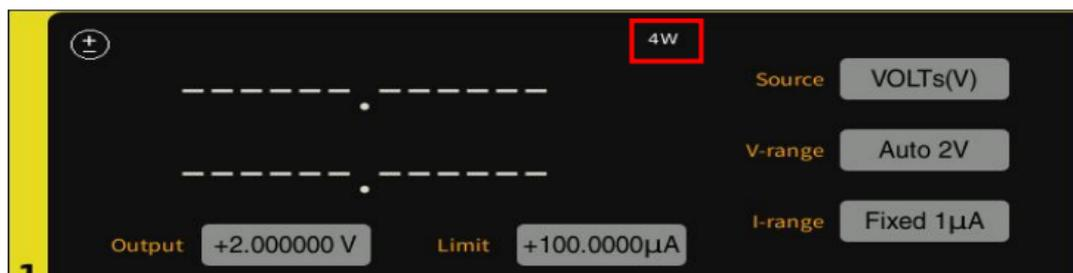
Figure 4-4 Connected 4-Wire Page Display Status
