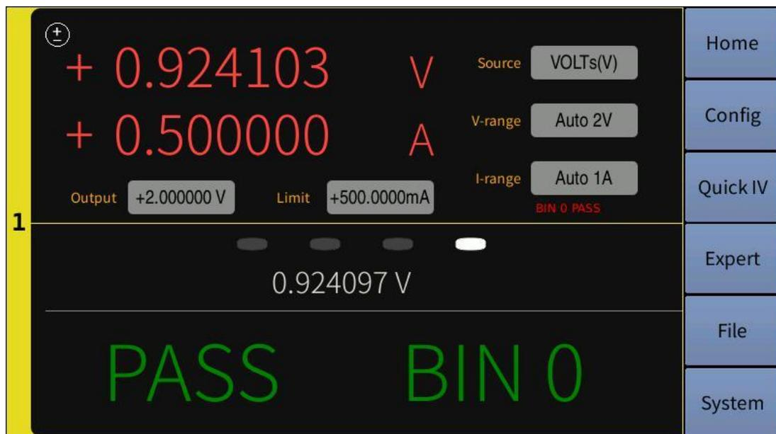
Figure 4-12 Channel Specific Setting Page 4 - Limit Test Status
