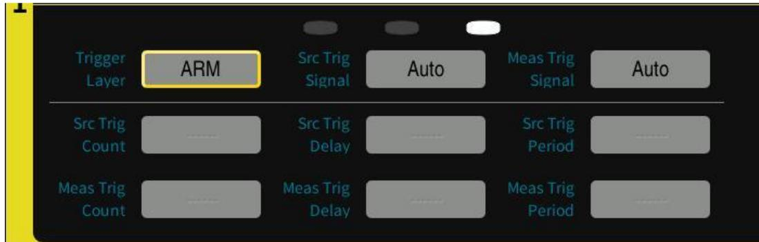
Figure 4-10 Channel Specific Setting Page 3 - ARM Trigger Layer
