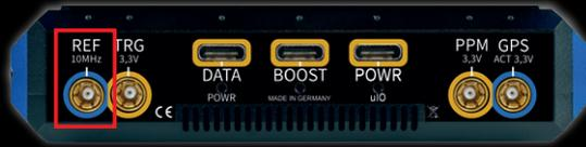
One SMB input labeled REF to connect an external 10 MHz clock signal.
