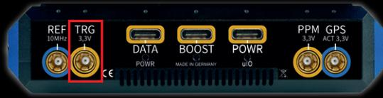
One SMB in/output labeled TRG for synchronizing device.
