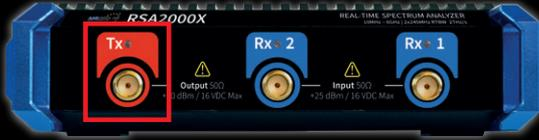
One SMA output labeled Tx to connect receiving equipment providing signal strengths of up to +20 dBm (not supported on RSA 250X).
