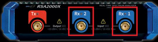
Two SMA inputs labeled Rx1 and Rx2 to connect antennas, generators or other measurement equipment supporting signal strengths of up to +25 dBm (Rx2 only supported on RSA 2000X).
