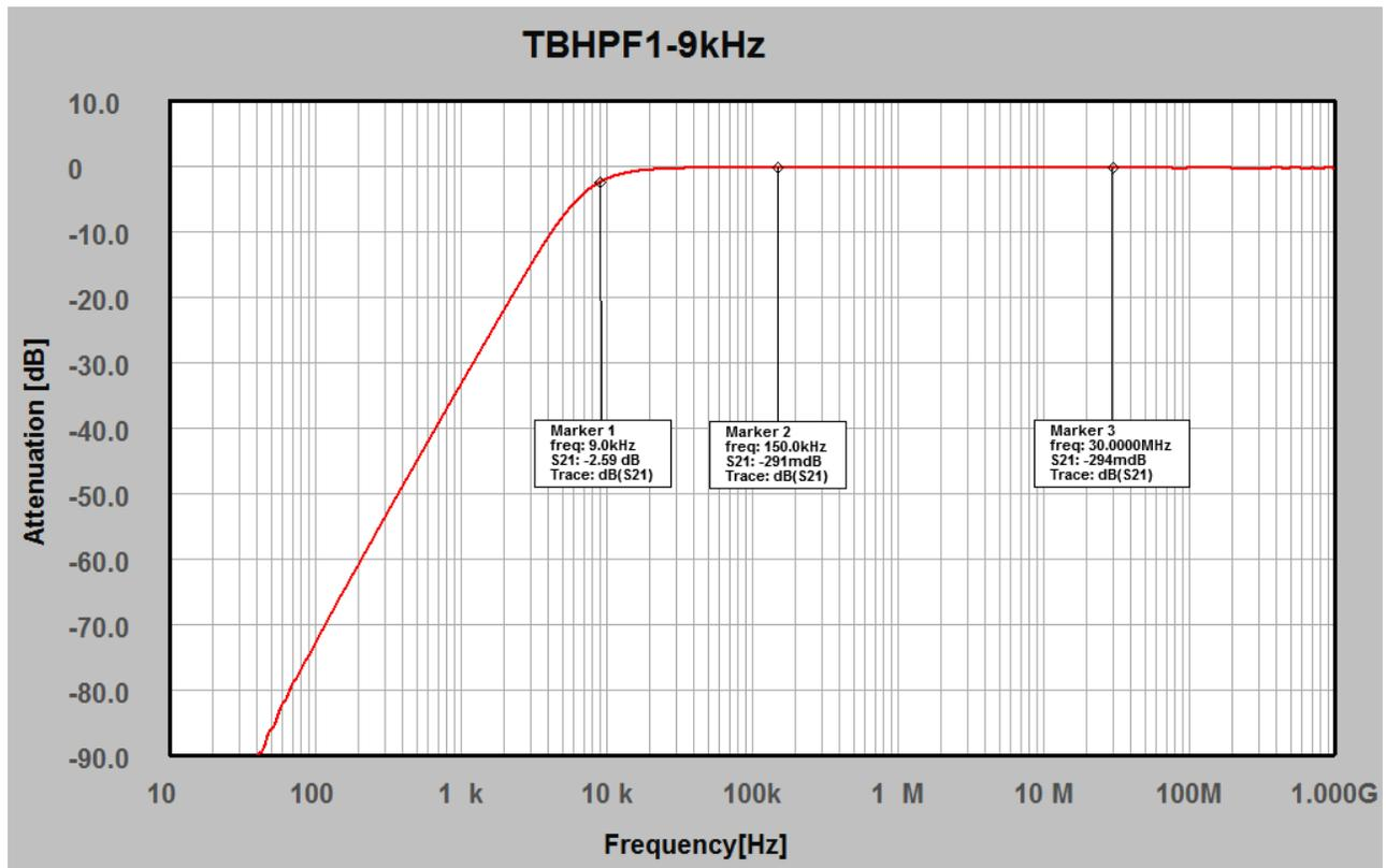
TBHPF1-9kHz: Attenuation 30 Hz to 1 GHz, typical data
