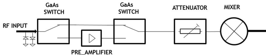
The diodes at the input typically serve as ESD protection diodes. In order to fully protect the input with a limiter, shunt diodes would need to be combined with a series resistor to limit forward current in case of excessive input signal. Consequently, a classic current limiting resistor solution cannot be implemented, as it would increase the input impedance of the analyzer.
