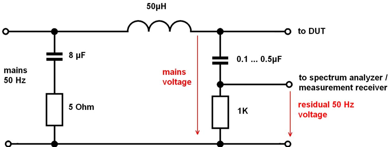
The full AC mains voltage is present at the DUT terminals of the LISN. The RF coupling capacitor and the 1K resistor form a voltage divider, which determines the amplitude of the 50 Hz voltage at the RF connector.
