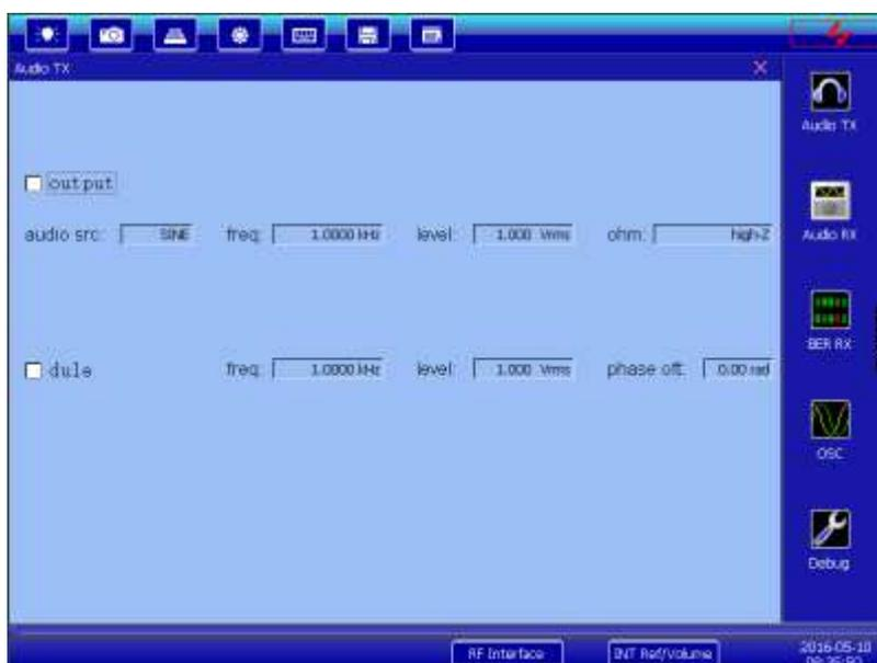
Fig. 3-12 Audio frequency generation interface
