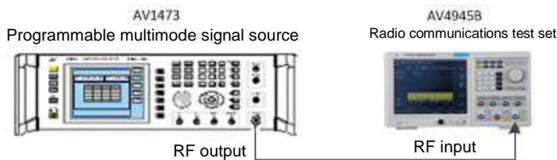
Fig. 4-9 Wiring diagram for sweeping spectrum measuring
