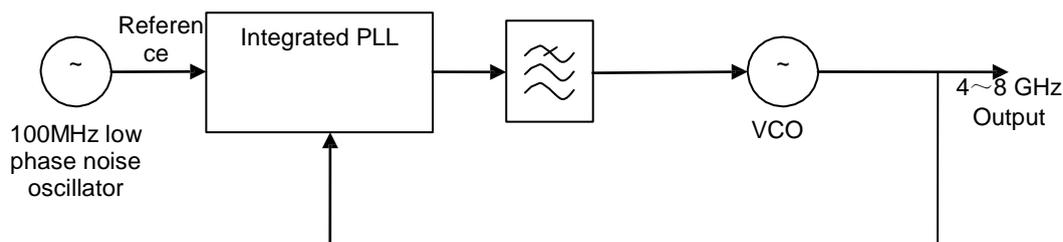
Fig. 5-5 Schematic diagram of local oscillation generation
