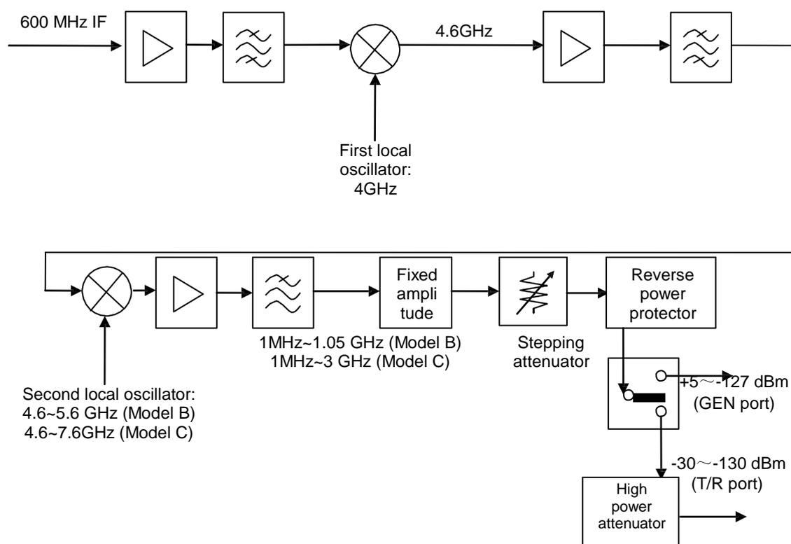
Fig. 5-3 RF conversion scheme of the transmitter
