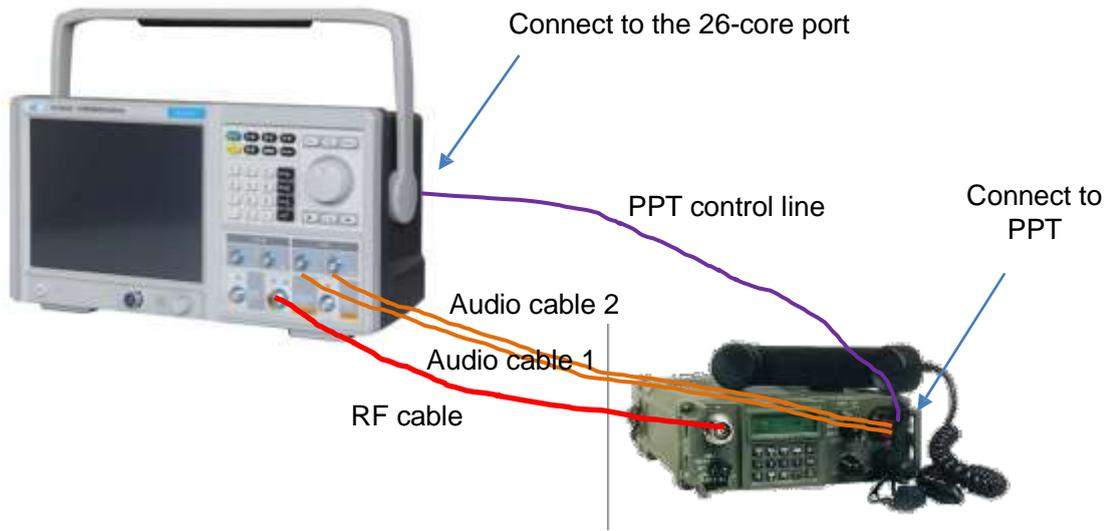
Fig. 4-21 Typical one-click auto test connection diagram
