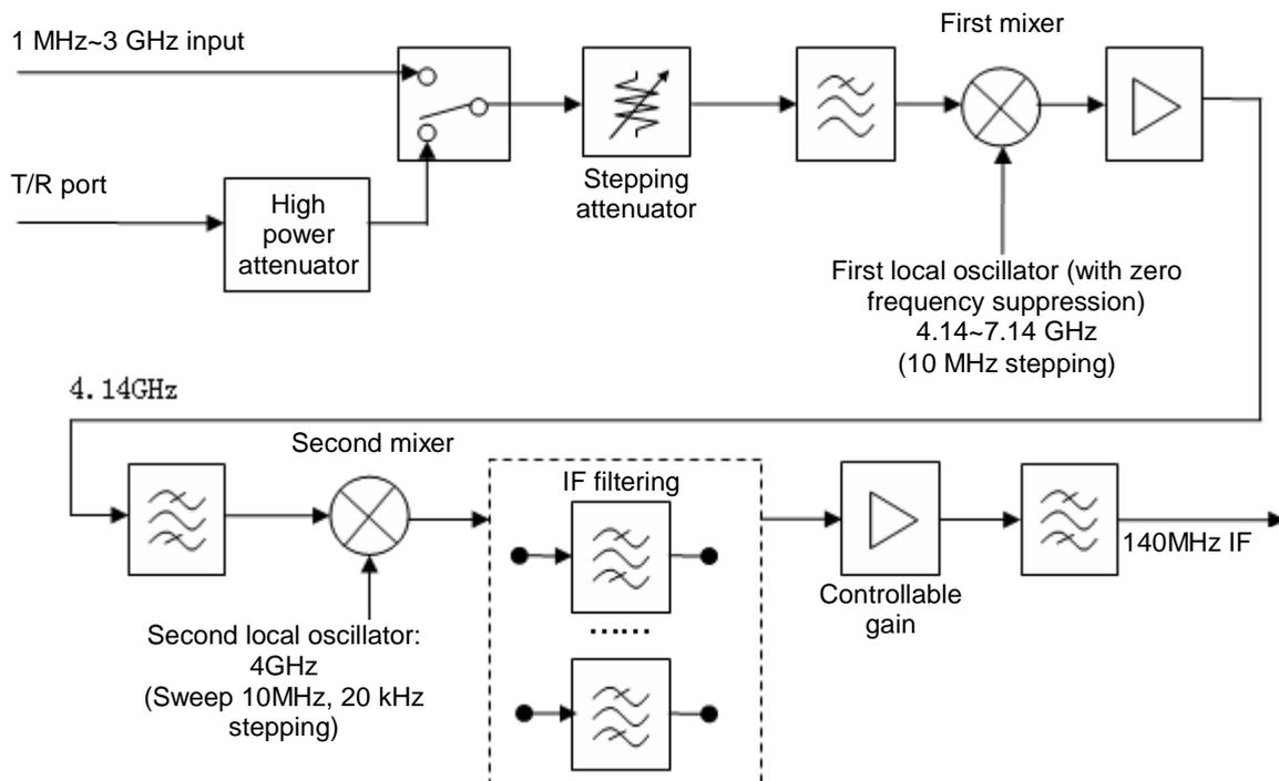
Fig. 5-4 RF conversion scheme of the receiver
