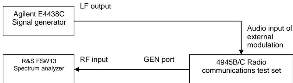
Fig. 6-9 Block diagram for external analog modulation characteristics test of RF signal generation
