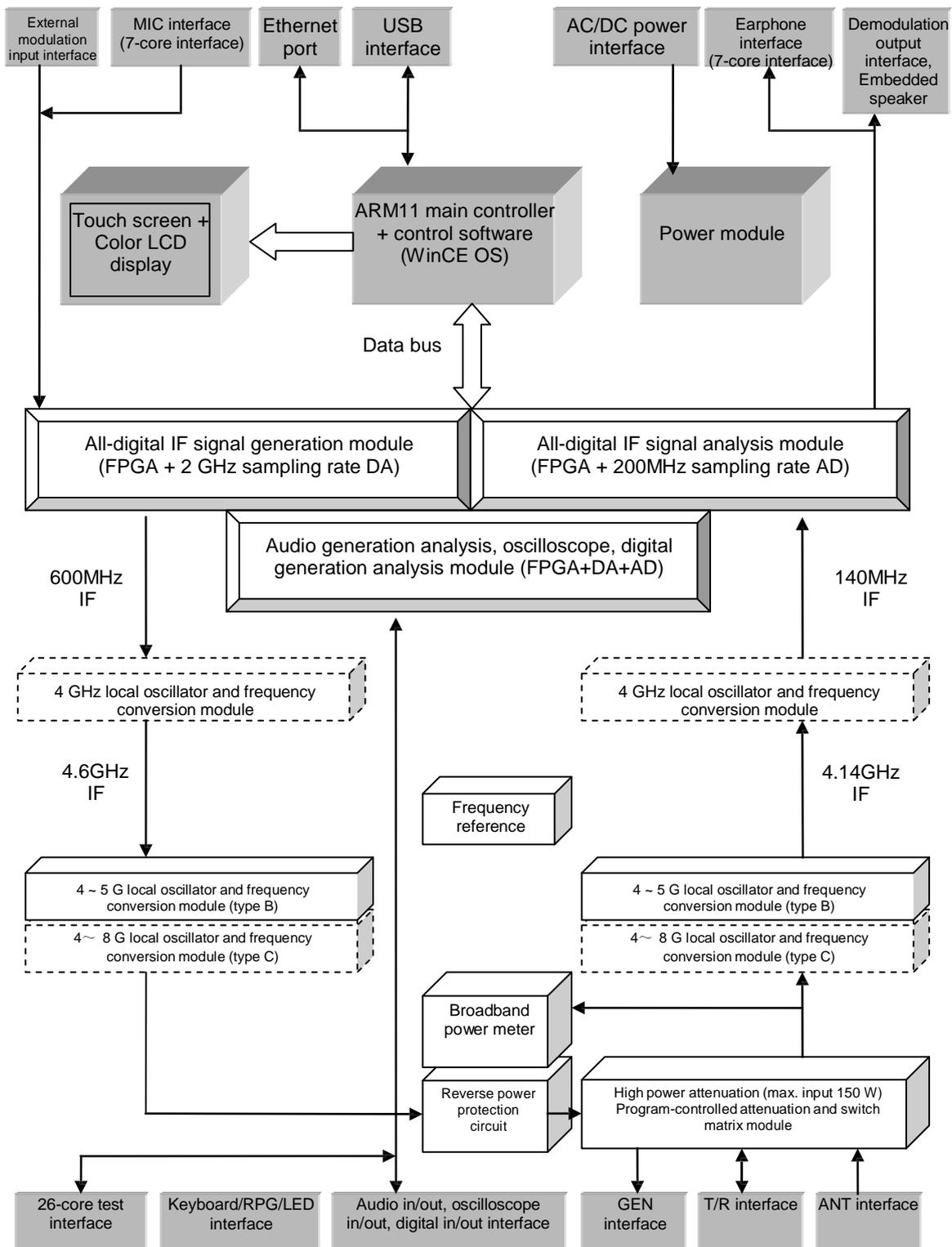
Fig. 5-1 Hardware block diagram of 4945B/C radio communications test set
