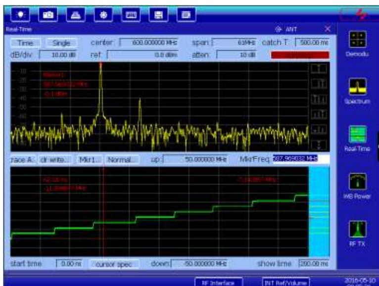
Fig. 4-12 Real-time spectrum analysis interface
