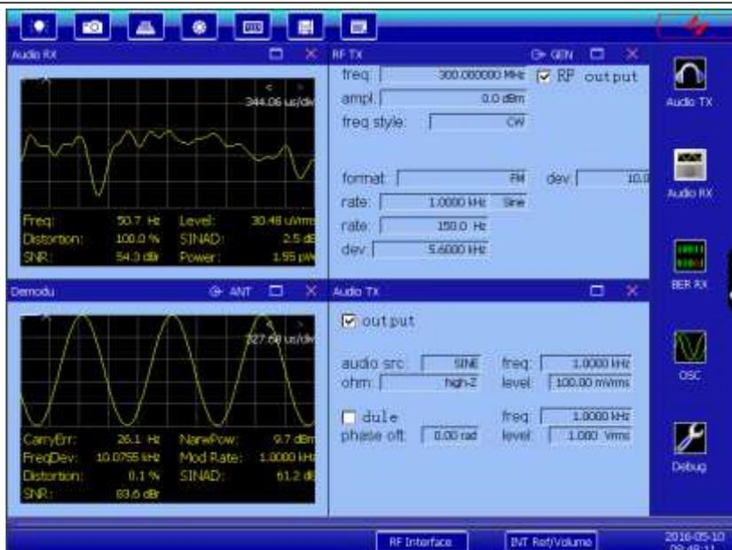
Fig. 3-19 Combined interface: RF emission, RF receipt, audio generation and audio analysis
