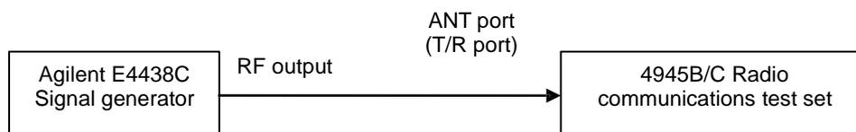
Fig. 6-2 Block diagram for RF RX and sweep spectrum characteristics tests
