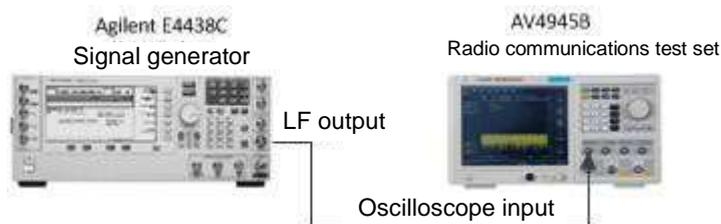
Fig. 4-17 Oscilloscope function connection diagram
