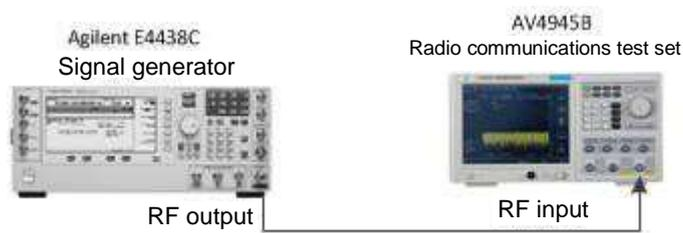
Fig. 4-5 RF receiver wiring diagram
