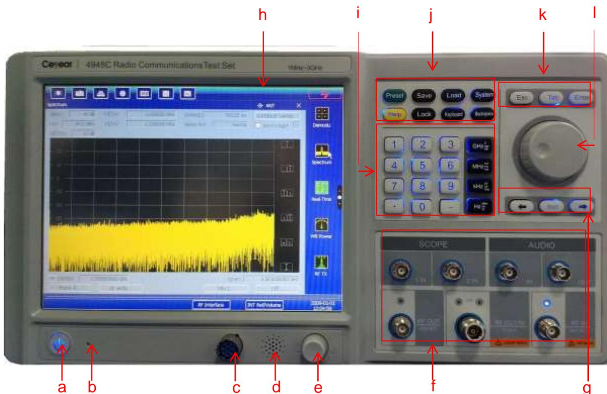
Fig. 2-2 Front panel schematic diagram of the 4945B/C radio communications test set
