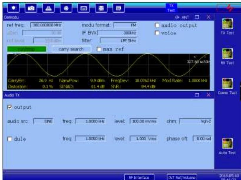
Fig. 3-18 Combined interface: RF receipt and audio generation
