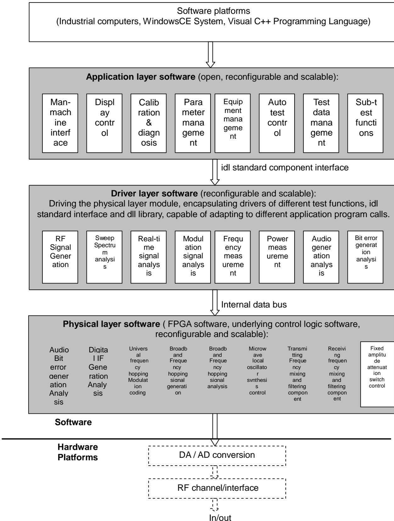
Fig. 5 -2 Overall software solution based on software radio
