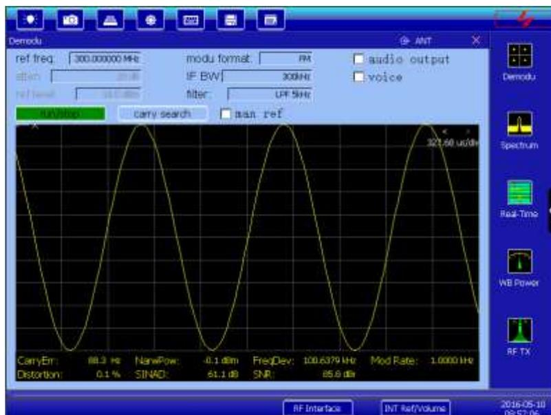
Fig. 4-6 FM demodulation interface
