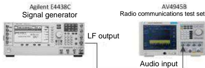
Fig. 4-14 Audio analyzer connection diagram
