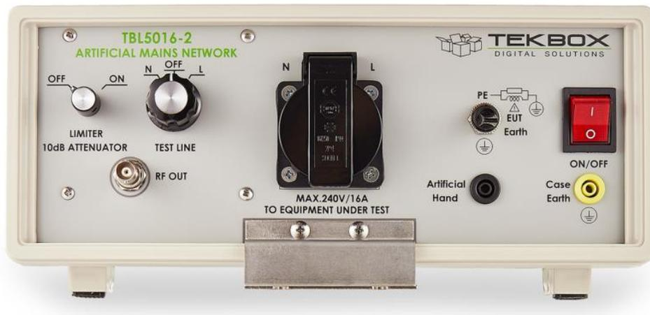
The TBL5016-2 is a Line Impedance Stabilization Network for the measurement of conducted emissions within the range of 9 kHz to 30MHz, according to the CISPR 16 standard. The device is designed for testing single phase, AC-powered equipment with supply voltages up to maximum of 240V. Conducted noise can be measured on the phase and on the neutral conductor. The TBL5016-2 is equipped with a switchable limiter/attenuator and an artificial hand connection.
