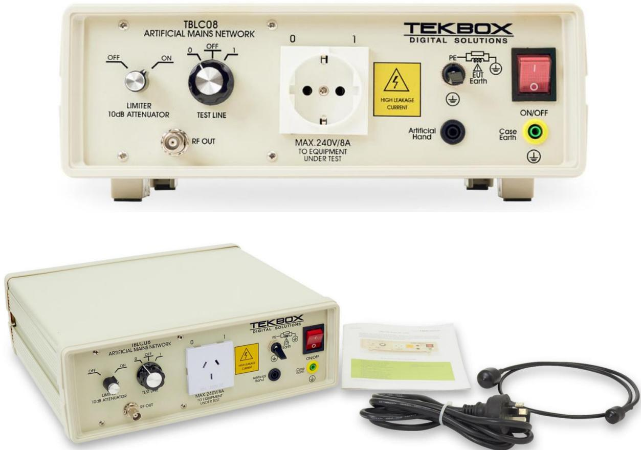
The TBLC08 is a Line Impedance Stabilization Network for the measurement of conducted emissions within the range of 9 kHz to 30MHz, according to the CISPR 16 standard. The device is designed for testing single phase, AC-powered equipment with supply voltages up to maximum of 240V. Conducted noise can be measured on the phase and on the neutral conductor. The TBLC08 is equipped with a switchable limiter/attenuator and an artificial hand connection.
