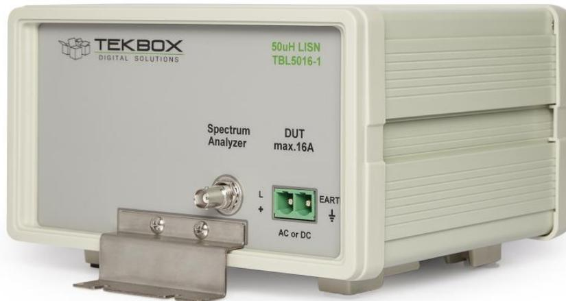
The TBL5016-1 50 $\mu$ H LISN is a versatile device for measuring conducted noise of DC, AC single phase or 3-phase powered electronic equipment. It is designed according to CISPR 16-1-2 and MIL-STD-461F standard and characterized in the frequency range of 9 kHz to 100 MHz.
