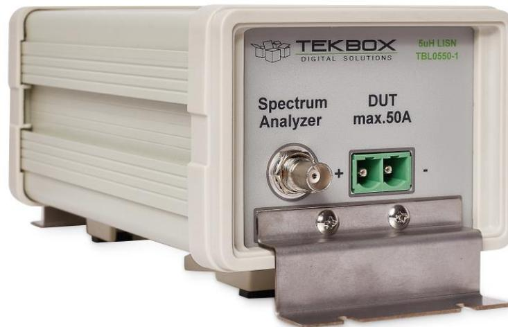
The TBL0550-1 5 $\mu$ H LISN is designed to be used for measurements in the frequency range of 150kHz to 110 MHz according to CISPR 16-1-2, CISPR-25, EN55025, MIL-STD-461F, ISO11452-4 and with limitations DO-160/ED-14G and ISO 7637-2.
