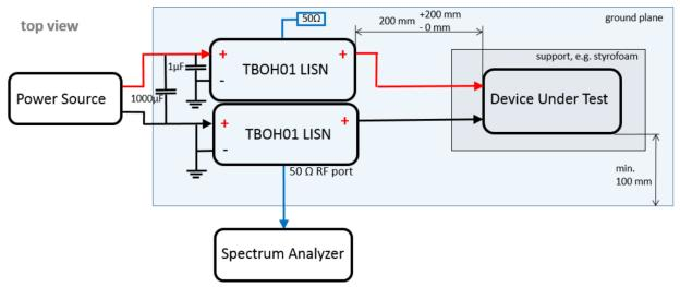
CISPR 25, voltage method, EUT (DUT) remotely grounded
