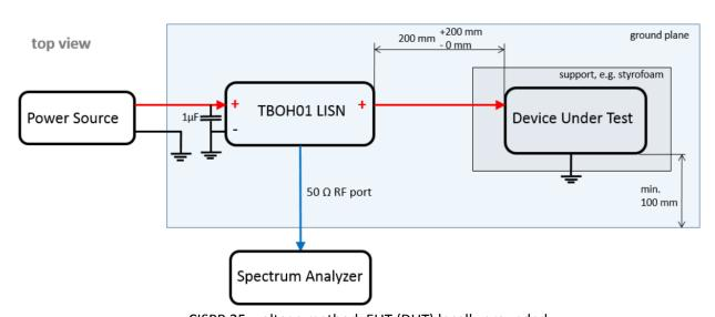
CISPR 25, voltage method, EUT (DUT) locally grounded
