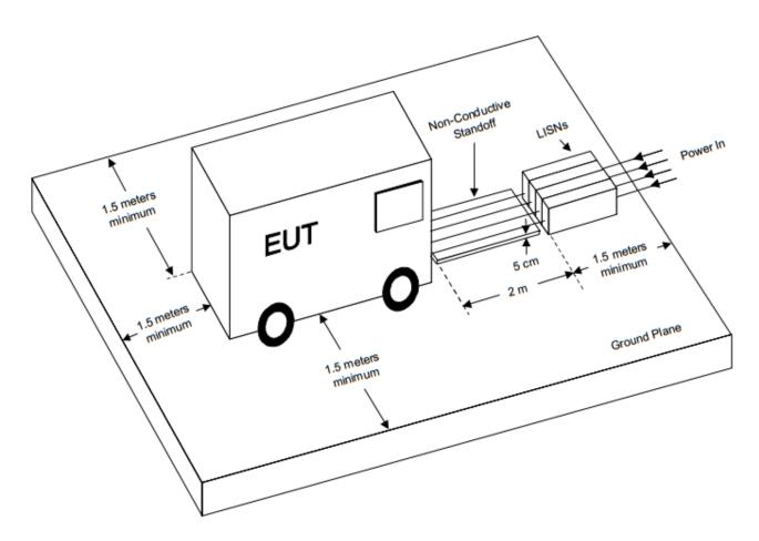
MIL-STD-461F test setup for free standing EUT
