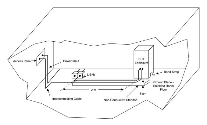
MIL-STD-461F setup for free standing EUT in shielded enclosure
