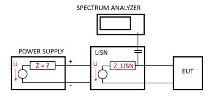
A LISN can be connected to any power supply and provide the same voltage and current capability as the power supply at the EUT terminals. However, the source impedance of the LISN is specified by EMC standards and enables repeatable conducted emission measurements in any laboratory.
