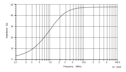
Figure E.1 - Characteristics of the AN impedance
