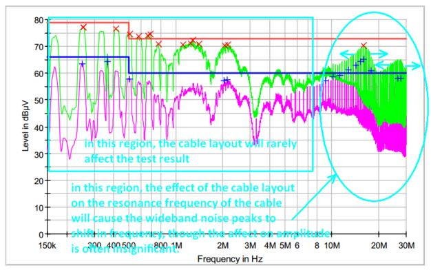
Effect of the cable layout on measurement results
