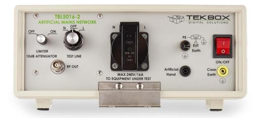
The TBL5016-2 is a Line Impedance Stabilization Network for the measurement of conducted emissions within the range of 9 kHz to 30MHz, according to the CISPR 16 standard. The device is designed for testing single phase, AC-powered equipment with supply voltages up to maximum of 240V. Conducted noise can be measured on the phase and on the neutral conductor. The TBLC08 is equipped with a switchable limiter/attenuator and an artificial hand connection.
