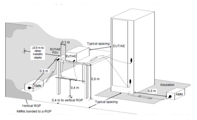
Set up for combination equipment
