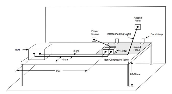
MIL-STD-461F setup for non-conductive surface mount EUT
