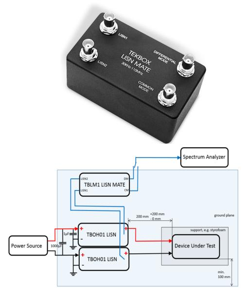
Measurement of differential mode and common mode conducted noise
