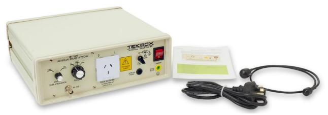
The TBLC08 is a Line Impedance Stabilization Network for the measurement of conducted emissions within the range of 9 kHz to 30MHz, according to the CISPR 16 standard. The device is designed for testing single phase, AC-powered equipment with supply voltages up to maximum of 240V. Conducted noise can be measured on the phase and on the neutral conductor. The TBLC08 is equipped with a switchable limiter/attenuator and an artificial hand connection.
