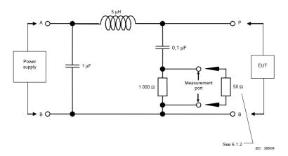
Figure E.2 – Example of 5 μH AN schematic
