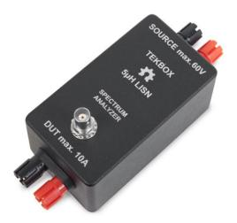
The TBOH01  $5\mu H$  LISN is designed to be used for EMC pre-compliance testing in the frequency range of 150kHz to 110 MHz according to the CISPR-25 standard, ISO 7637-2, ISO11452-2/4/5 and with limitations DO-160/ED-14G.
