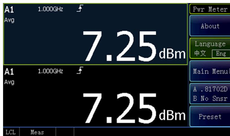
When the peak power sensor is connected, it becomes high-performance peak power meter. The amplitude and time domain parameters of pulse modulated signals in 50MHz ~ 67GHz band can be measured and analyzed.
