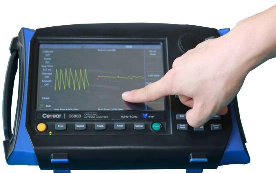
Finger sliding to switch measurement types
