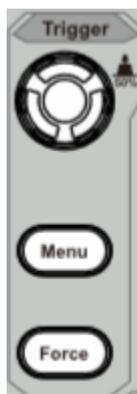
Figure 3-12 Trigger Control Zone
