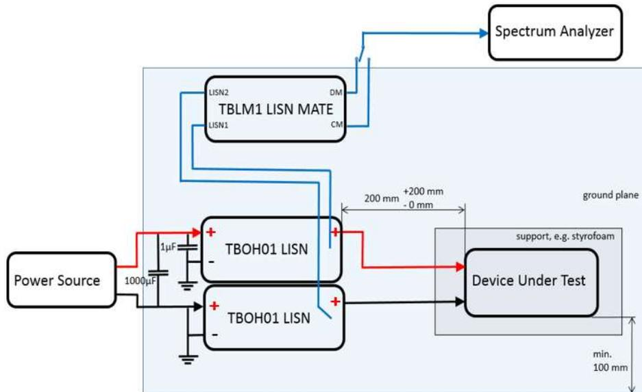
Picture 2: set up for the measurement of differential mode and common mode conducted noise
